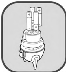
4. Insert 4 x AA batteries making sure that the flat end of each battery (negative) touches the contact spring.
