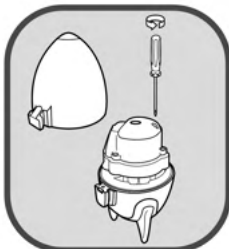
3. Undo the battery compartment screw and remove lid.
