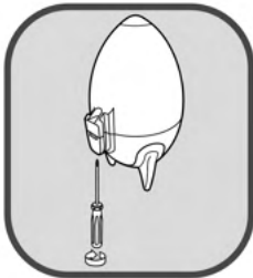
1. Undo retaining screw. (Screw will not fall out).
