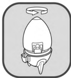
2. Twist to unlock top casing and remove.
